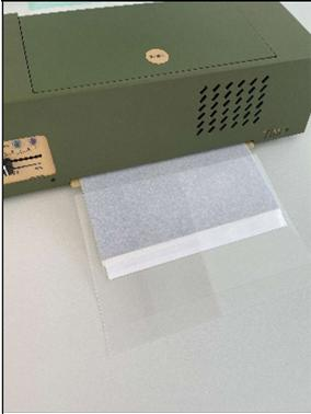
Set a medium speed on the feed controller of the cold unit.
